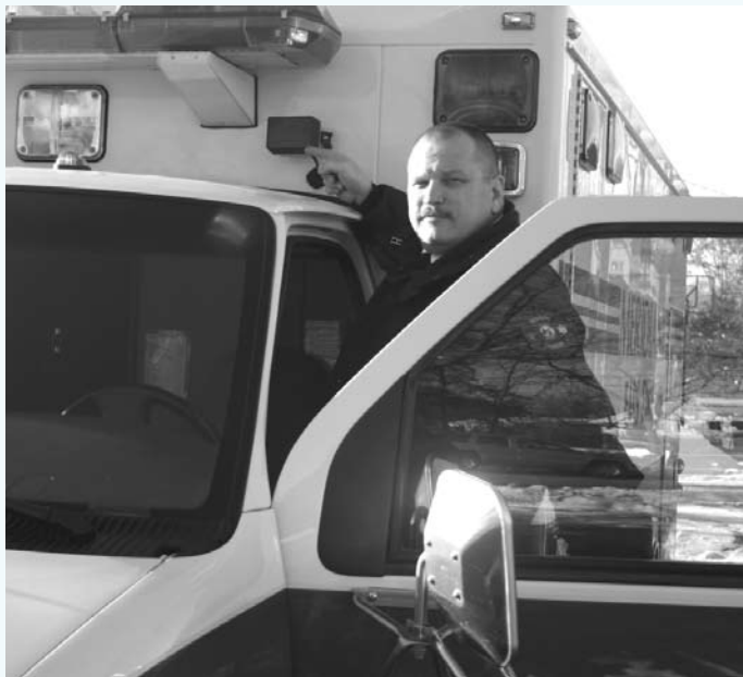
EMS Coordinator Greg Hammond points to the infrared sender unit mounted near the top of the ambulance.
